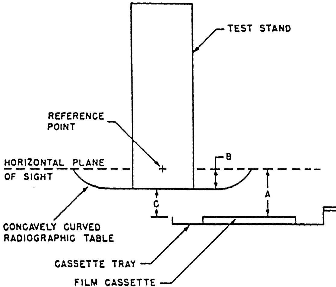
FIGURE 1: HOW TO DETERMINE DISTANCE FROM TOP CASSETTE TO BASE OF TEST STAND FOR CONCAVELY CURVED TABLE TOP.
