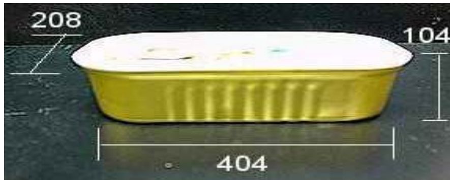
Figure 18 – Measurement of a Low-Profile Container
