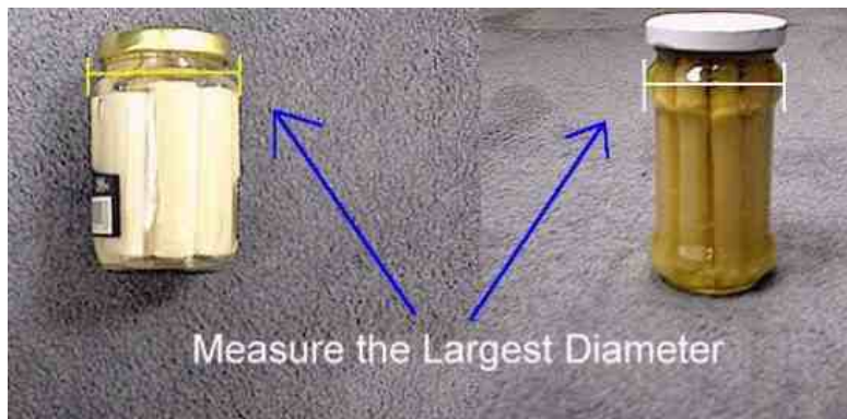
Figure 16 – Measurement of an Unusual Shape Cylindrical Container.
