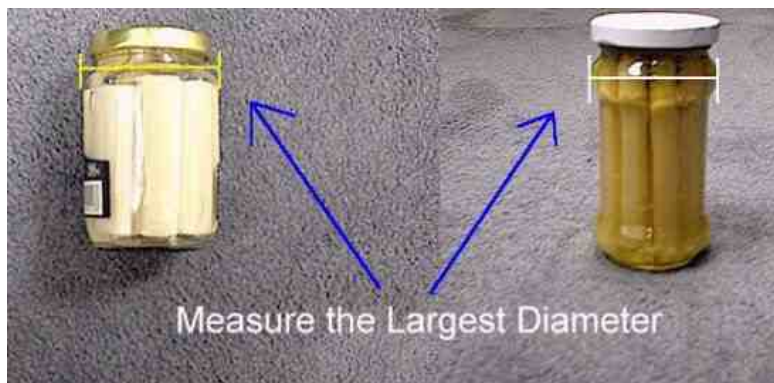
Figure 42 – Measurement of an Unusual Shape Cylindrical Container.
