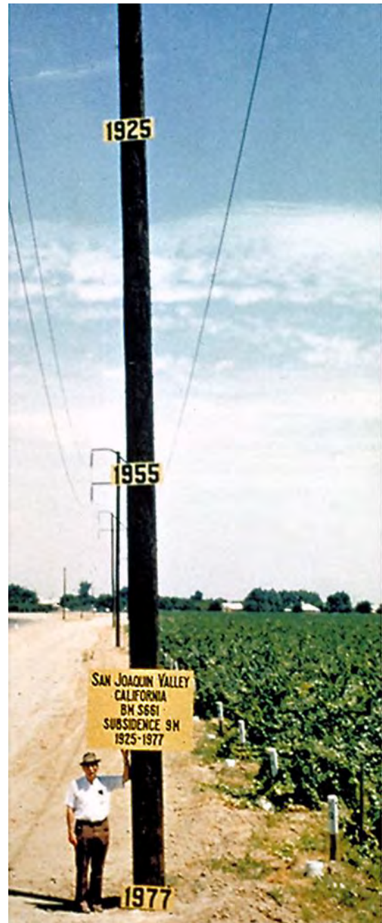
Figure 3.3-13. Example of soil subsidence as a result of aquifer compaction (Photo credit: Dick Ireland, USGS)
