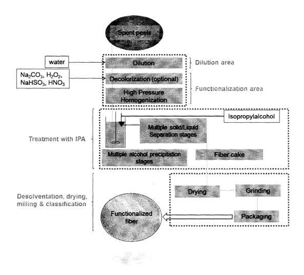
Spent peels are transferred from the pectin manufacturing site to the spent peels buffer tank. The first step in the manufacturing process (conducted in the dilution tank) is to hydrate the spent peels and reduce the dry substance of the spent peels (ds) to  $\leq 6\%$ . Seeds and other large materials are removed from the hydrated peels and discarded.
