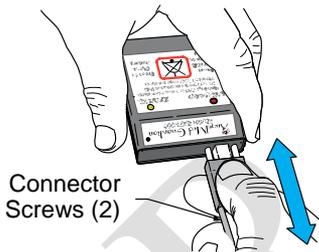
***To connect/disconnect the EXD Cable to/from the Programmer:***
