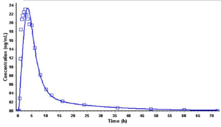
Plasma Concentration *versus* Time Profile Simulated (line) using Theoretical pH Solubility Profile *versus* Observed (empty squares)
