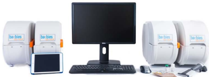
Figure 6: A high throughput workstation consists of 4 SEEKER™ analyzers connected to a central computer workstation.
